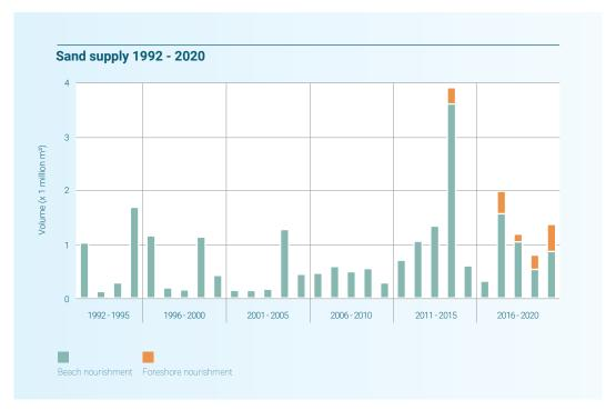
**Figure 3.** Evolution of the annual volumes of sand for beach and foreshore nourishment (Source: Coastal division). In the case of a beach nourishment, sea sand is applied via dredgers above the low-water line. For forshore nourishment, the sand is applied below the low-water line.
